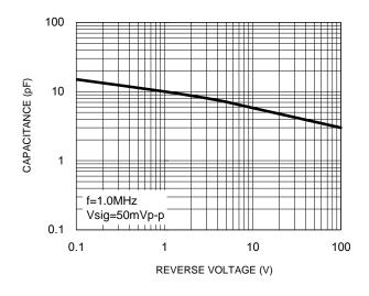
Fig.2 Typical Junction Capacitance
